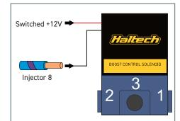
Example wiring connection using a spare injector output to digitally pulse a boost control solenoid.
