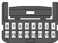
AUXILIARY CONNECTOR (16 PIN) REAR VIEW (WIRE SIDE)
