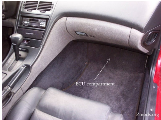
Figure 2 - Factory ECU Location
