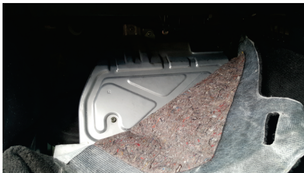
Figure 1 - Remove the panel by removing 4 nuts using a 10mm socket.
