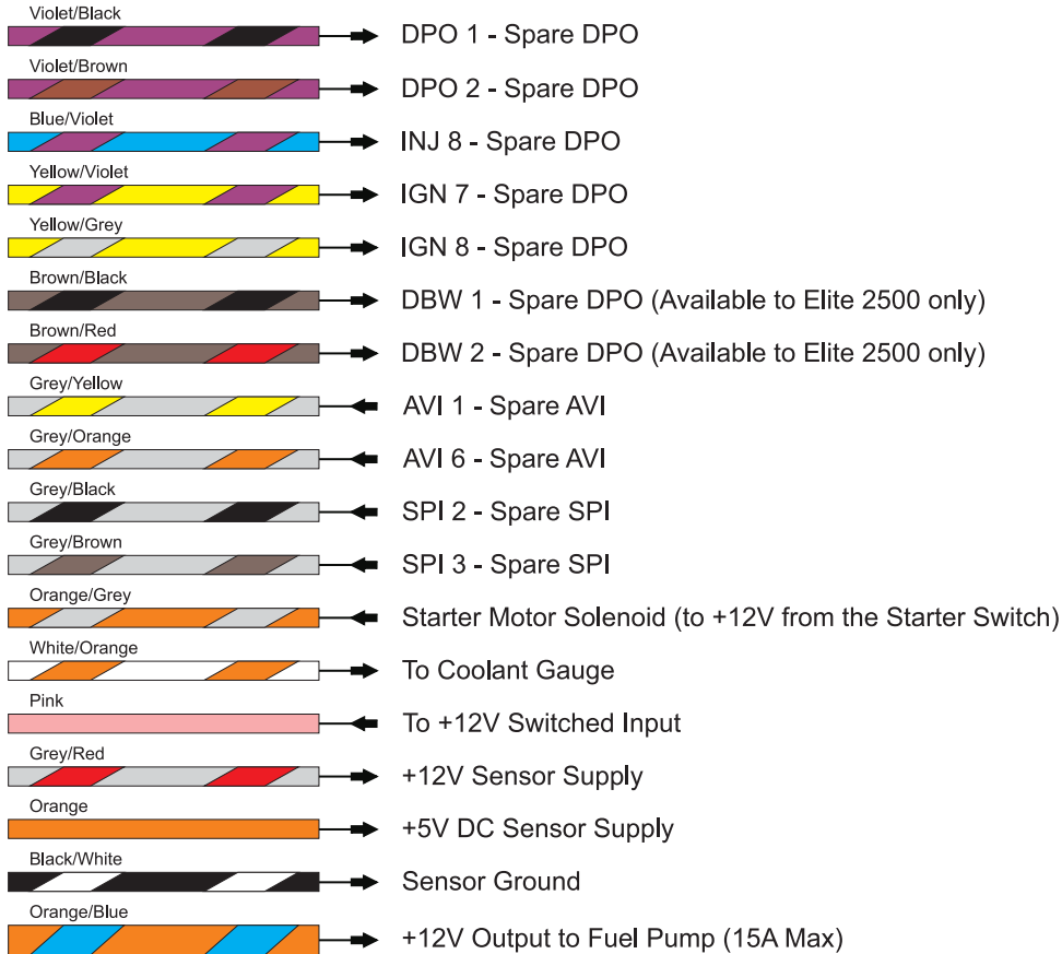
Figure 8 - In Cabin Harness Wiring
