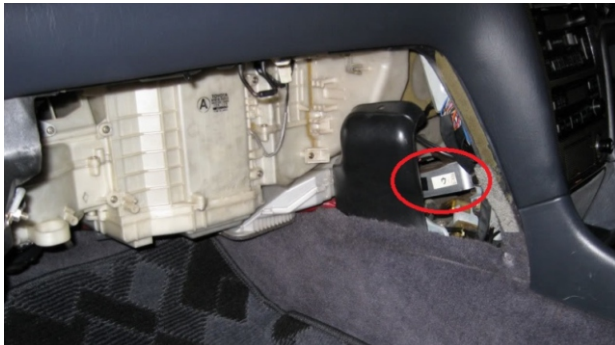
Figure 1 - JZX100 ECU Location
