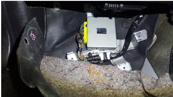
Figure 3 - Factory ECU is now ready for removal.
