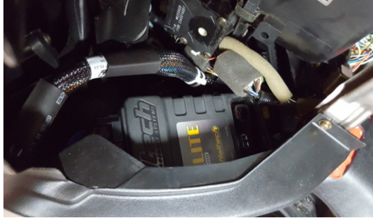
Figure 2 - Installation of Haltech Elite ECU
